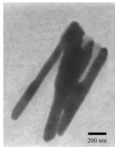
Figure 3 TEM images of ZnO nanorods after sintering.
